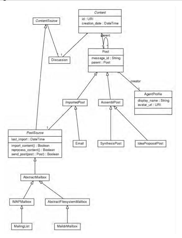
Figure 1: Assembl simplified diagram (processing of posts)
